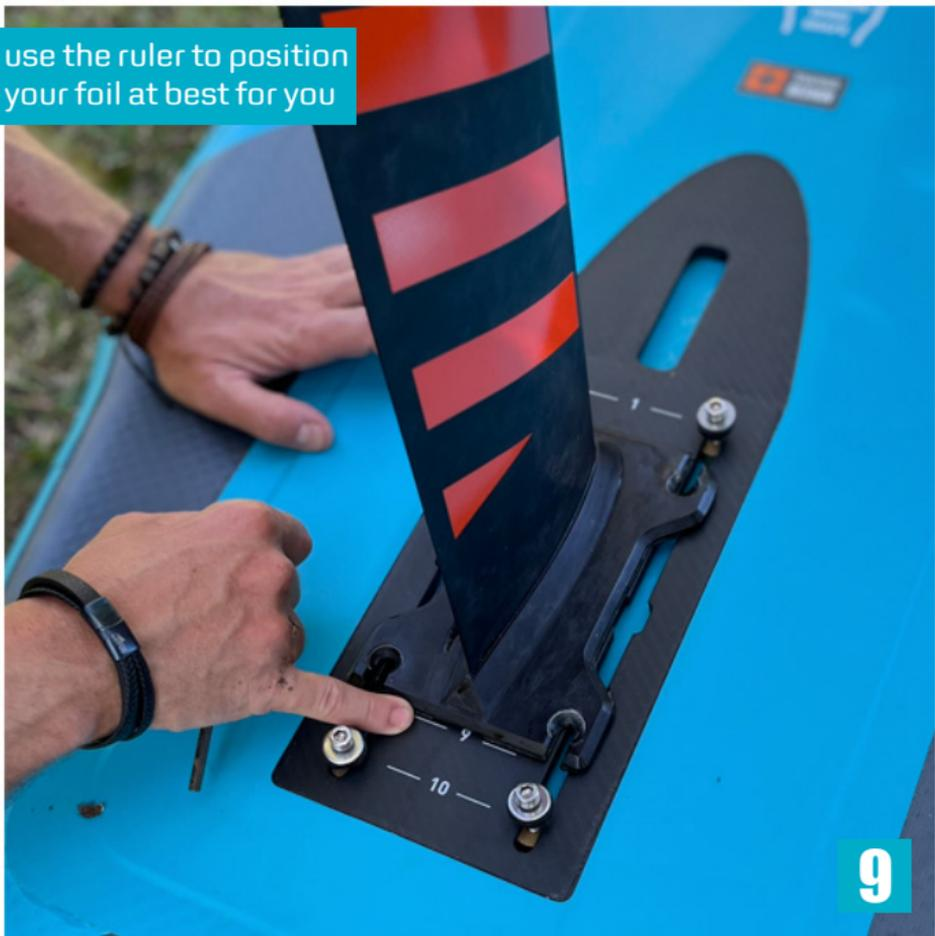
depending your kind of foil. the extra rubber device can be useful for an optimal tightening
